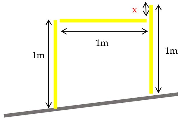
Figure 5.4 Illustration of the use of metre sticks and a spirit level to determine fall in gradient on a raised bog. Slope is determined by dividing the difference in height (x) by the length (1m in this case) (adapted from [www.ipcc.ie](http://www.ipcc.ie))
