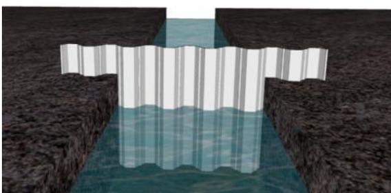
6. If significant flow is expected create a notch in the dam
