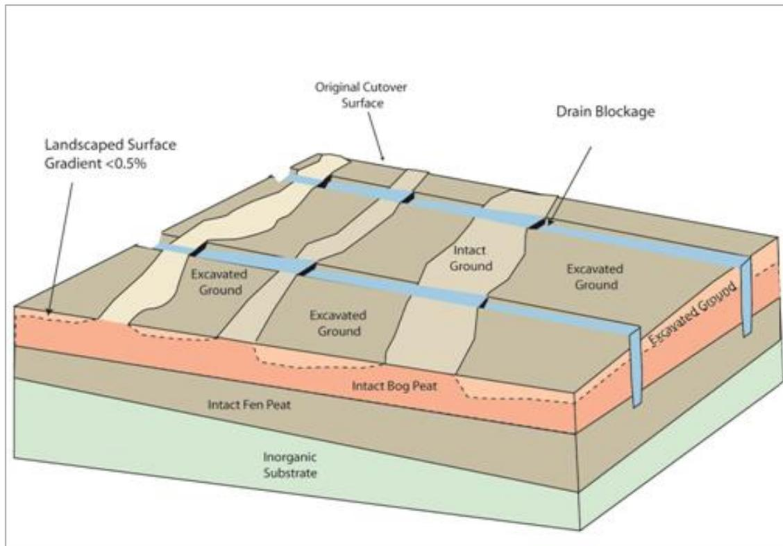
Figure 5.13 Schematic illustrating excavation and re-profiling of cutover bog to create suitable hydrological conditions for establishment of peat-forming habitats
