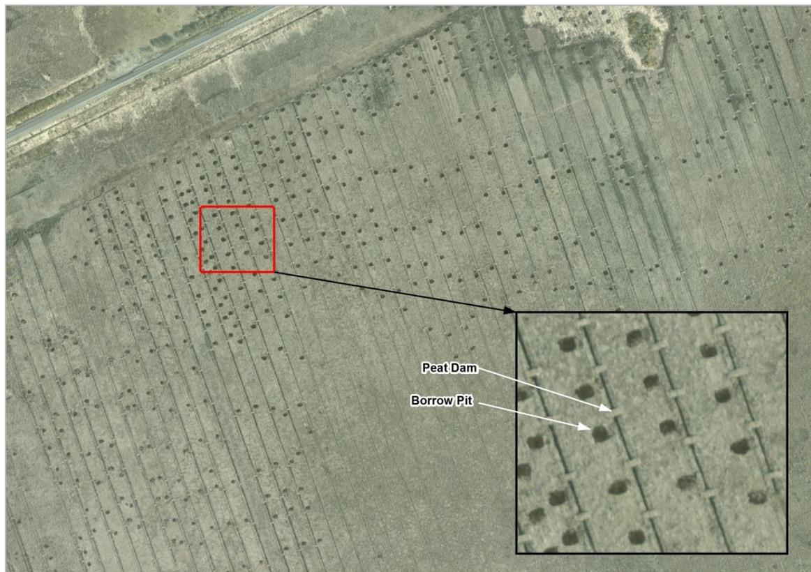
Figure 5.3 Aerial photography (2014) illustrating extensive high bog drain blocking at Ballydangan Bog, Co. Roscommon
