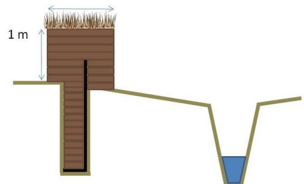
6. Completed marginal bund with weir overflow and bank protection for embankment
