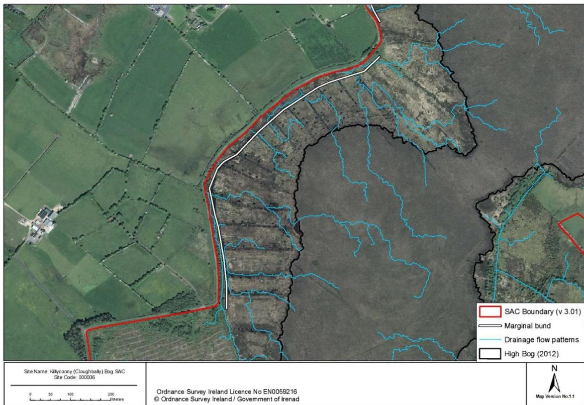
Figure 5.9 Location of marginal bund at Killyconny (Cloughbally) Bog SAC. Note the simulated drainage patterns indicate significant flow from the high bog flows towards the western margin
