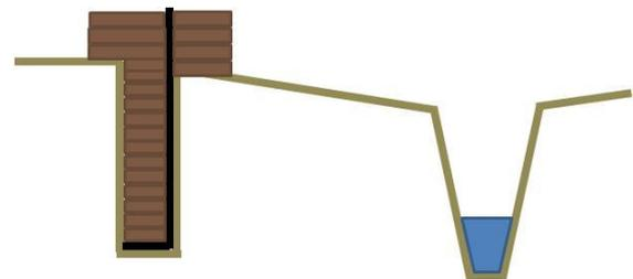
5. Build up layers of compacted peat, place scraw on top and sides of completed embankment
