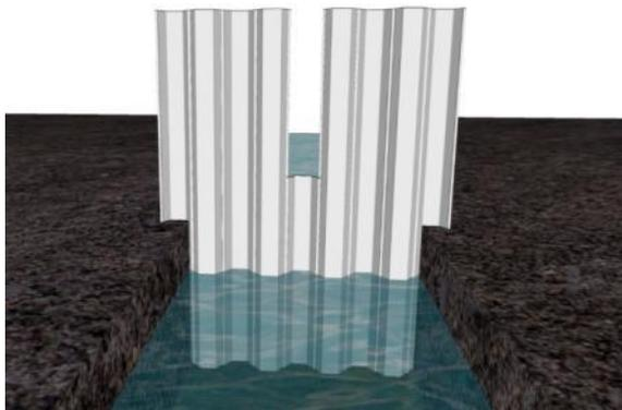
4. Ensure dam extends into bog by minimum of 50cm
