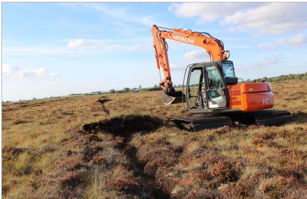
Figure 5.16 Machine currently used by Bord na Móna to block drains on the high bog (Hitachi Zaxis 70LC) © David Fallon (Bord na Móna)
